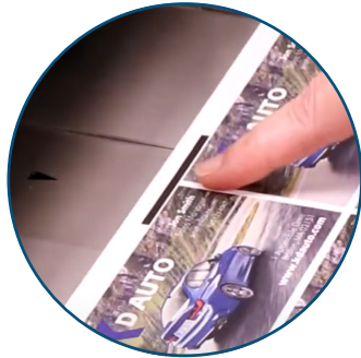
Cut-Mark Sensor Reads any image drift, then registers to ensure consistent finishing
