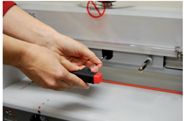
Blade change safety tool in place
