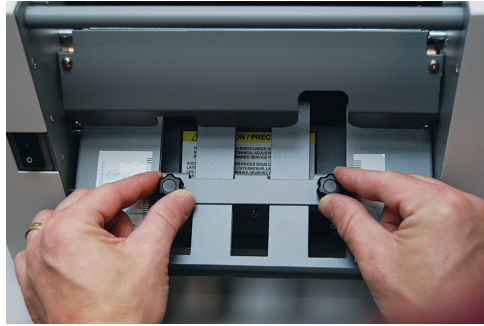
Fig. 2b Adjusting lower fold plate
