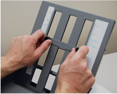
Fig. 2a Adjusting upper fold plate
