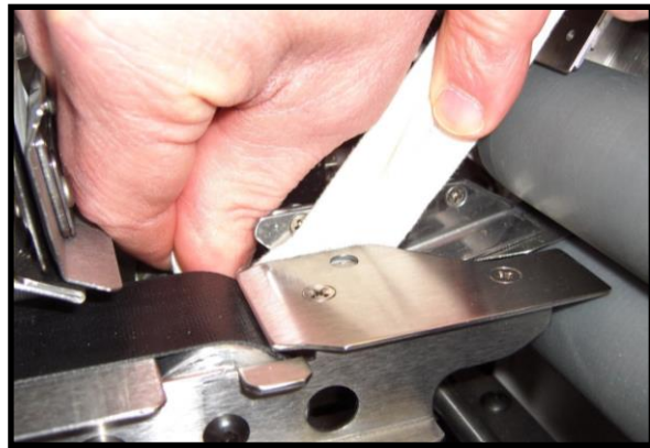
Cleaning the Tab Wrap Guide Located at the exit end of the Left Media Guide Assembly.
