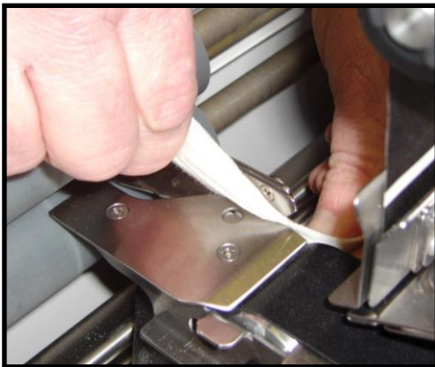
Cleaning the Tab Wrap Guide Located at the exit end of the Right Media Guide Assembly.
