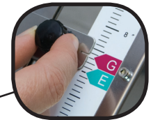
Align the fold stop notch with the matching letter.
