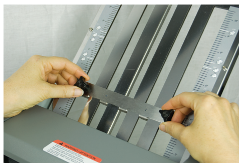
Loosen the thumbscrews to adjust the fold stop position.
