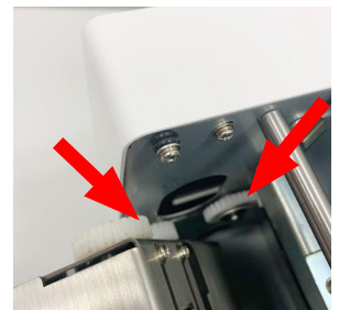
7. Align the gears on the blade cassette with the machine gears
