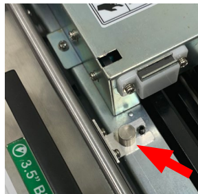
5. Remove thumb screw and remove blade cassette
