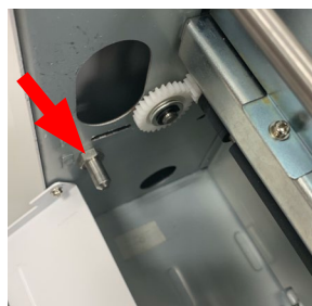
6b. Align blade cassette notch with mounting pin
